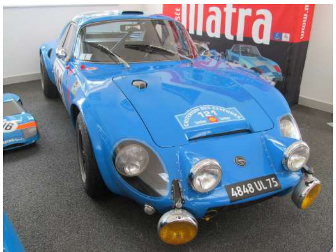
1965 Matra M610 rally car Cosworth Ford Twin Cam engine, Hewland gearbox, 645kg 145 bhp
